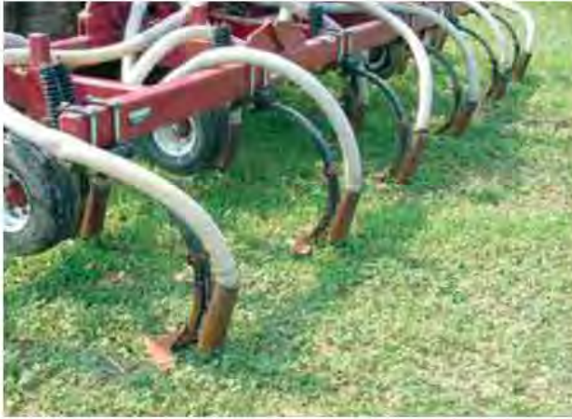
Figure 14.6. Equipment for manure injection with minimal soil disturbance.
