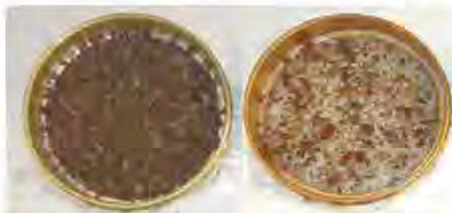
Figure 23.6. Results of an aggregate stability test for silt loam vegetable soils: organic (70% stable, left) and conventional (20% stable, right) management.
