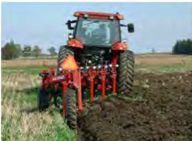
Figure 16.4. Left: Moldboard plowing inverts the soil and leaves no surface protection. Right: Chisel plow shanks loosen soil and leave some residue cover.
