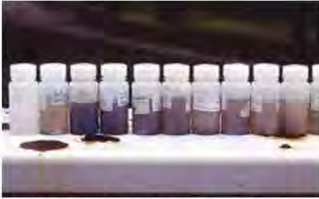
Figure 17.22. Water samples taken from a subsurface drain line when heavy rainfall followed liquid manure application. From left, water samples represent 15-minute sampling intervals from the onset of drain discharge. Photo by Larry Geohring.
